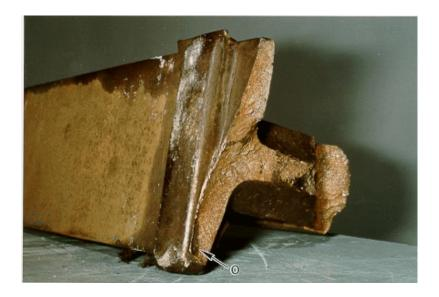
The two surfaces of the pre-crack were cut out of the east and west rail sections. Analysis of these pieces with a scanning electron microscope and a metallurgical microscope confirmed that the pre-crack had begun in an area of acicular ferrite, a microstructure that has less resistance to fracture and impact, and that there was no recent extension of the pre-crack.
