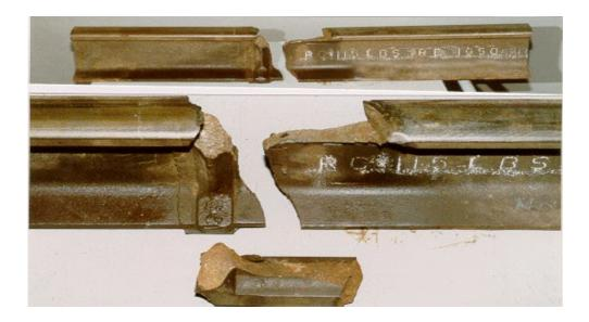
The rail east of the break had been rolled in 1950 and the one to the west, in 1979. Vertical wear and flange wear were within the acceptable limits set out in CN's SPC 3200 for 115-pound rail, namely 16 mm (5/8 inch) for vertical wear and 21 mm (13/16 inch) for combined vertical and flange wear.
