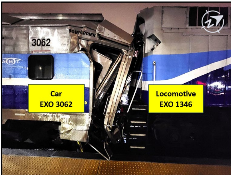
Figure 4. Damage to car EXO 3062 and the rear portion of locomotive EXO 1346 (Source: TSB)
