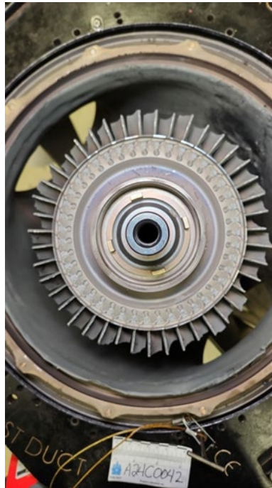
Figure 4. The occurrence aircraft's 2nd stage power turbine once removed from the engine with broken blades visible (Source: TSB)
