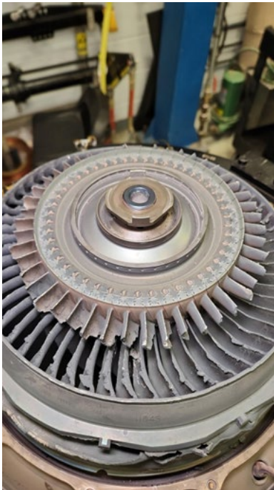
Figure 3. The occurrence aircraft's 1st stage power turbine once removed from the engine with broken blades visible (Source: TSB)
