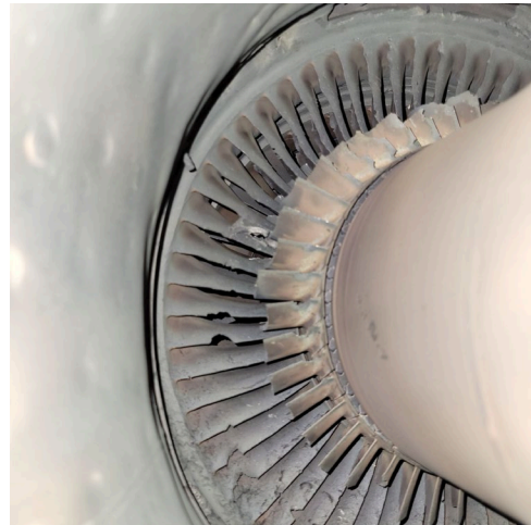
Figure 2. View of the occurrence aircraft's 2nd stage power turbine with broken blades when looking in through the exhaust duct (Source: TSB)
