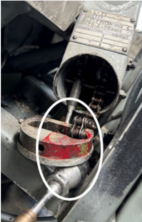
Figure 2. Red paint on the inner surface of the guide block at the base of the control column (Source: Third party, with permission, and with TSB annotations)
