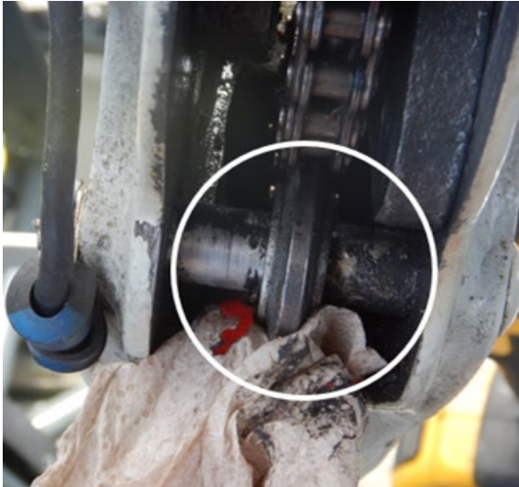
Figure 3. Red paint remaining on the chain guide at the control column pivot point once the grease was wiped off (Source: TSB)
