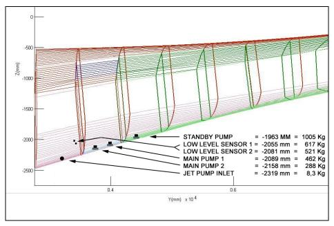
Figure 5. Inner fuel tank modeling (cross-section)
