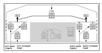
Figure 4. Fuel system controls
