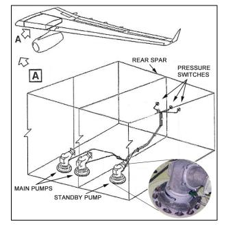
**Figure 2.** Fuel pumps and pressure switches
