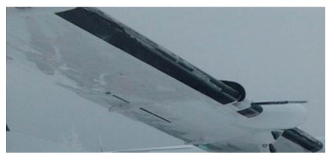
Photo 1. Ice on leading edge of wing before the accident flight
