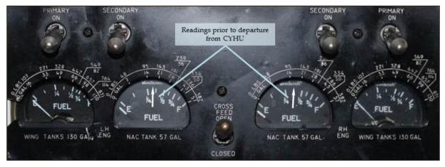
Figure 5. Illustration of the quantity of fuel before the occurrence flight
