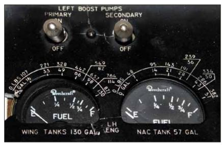
Calibration of the fuel gauges is not required, and no adjustment is called for in the aircraft maintenance manual. In the event that a gauge provides a faulty reading, the instrument is replaced.
