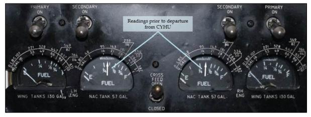
Further, although the fuel gauges of the wing tanks are similar to those of the nacelle tanks, the graduation scales of the 2 types of gauges differ. The "F" position on each fuel gauge dial represents 871 pounds in the wing tanks, but 382 pounds in the nacelle tanks. Similarly, the midpoint of the dial represents 310 pounds in the wing tanks, but 130 pounds in the nacelle tanks.
