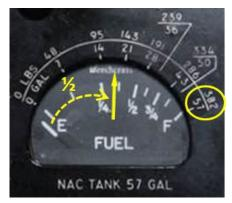
tanks completely full and the fuel gauge needles at the "F" position. Since the fuel consumption of both engines is generally similar, the quantity of fuel in the wing tanks can be determined by reading one of the wing tank gauges and multiplying that reading by 2.
