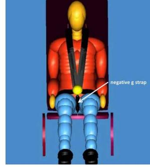
Figure 5. Example of a negative *g* strap (Source: Wichita State University)
