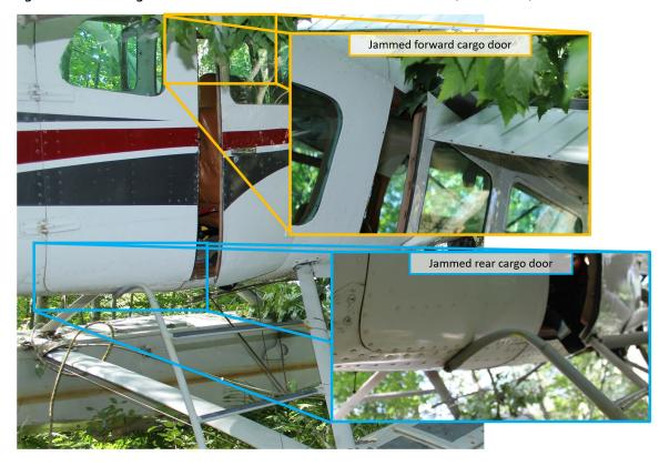
Figure 3. Double cargo door of the occurrence aircraft after the accident (Source: TSB)
