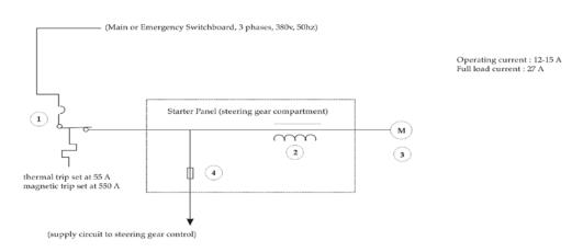
Electrical Arrangement of Steering Gear Power Unit and Control Circuits
