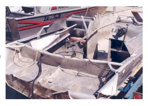
reported as being non-operational. Consequently, shipped water could not be discharged from the vessel. In the heavy rolling sea with cresting waves, the free-surface effect of the entrapped water on board would have contributed to the capsizing action.
