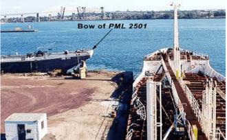
The *PML 2501* is a square-ended, non-propelled petroleum tank barge of steel construction. It was moored in a westerly direction along the southern end of the Algoma Steel Corporation wharf (see Photo 1).
