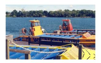
Seven rows of anti-shock, foam-cushioned and spring-dampened benches make up the passenger seating area. This area is fitted between moulded, compartmentalized buoyancy tanks, which also form part of the outer hull, sides and bottom. Immediately in front of each row of seating is a horizontal stainless steel support bar at arm's reach, grasped by the
