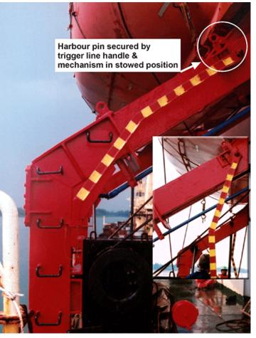
for the intended voyage, with the lifeboat stowed under the gravity davits in the "locked" position. However, the port side davit system was in the released condition, with the lifeboat held in place with only lashing lines and
