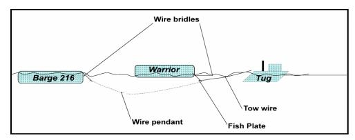
**Figure 1.** Towing arrangement for the tug *Ocean Warrior* and barges *Warrior* and *Barge 216*
