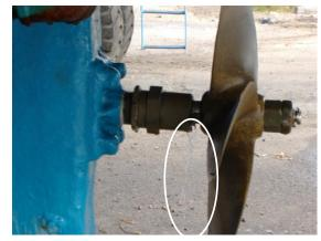
**Photo 4.** Leaking stuffing box after vessel recovery
