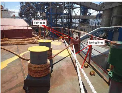
During their deployment, the 2 spring lines were initially kept loose between the dock and the vessel. At 1509, the pilot informed the master that the *Nord Quebec* was in position. The main engine was already stopped and the master ordered the second officer to heave on the spring lines to keep the vessel in place. The second officer relayed the order to the bosun and both spring lines were pulled taut with the port mooring unit, stopping the vessel's motion.
