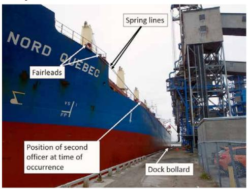
Figure 3. *Nord Quebec* alongside section 16 of Port of Trois-Rivières, Quebec, showing mooring configuration and location of bollard, fender, and forward spring lines following occurrence
