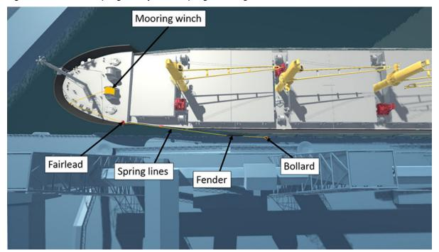
Figure 7. Illustration of spring line layout and spring lines caught under fender
