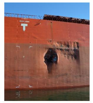
Figure 5. Damage to the *Caravos Harmony* (Source: TSB)
