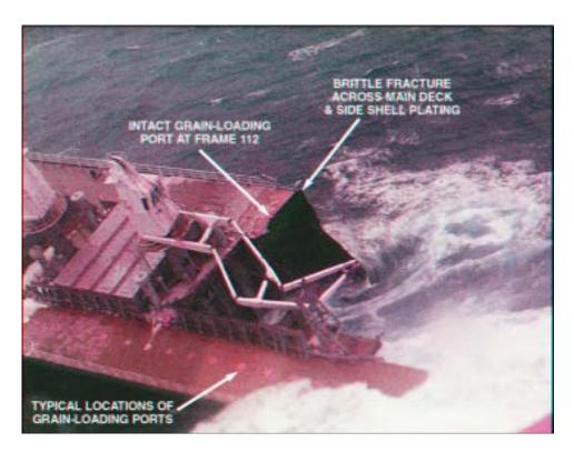
The depth of water was some 100 m, and the maximum length of the port side of the damaged hull was approximately 120 m. Consequently, the after port side was the first part of the wreck to come in contact with the seabed. Due to the heaving motions in the prevailing rough sea conditions, it sustained some impact damage in addition to that incurred during the hull separation.
