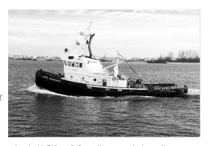
is approximately 7.5 knots. The vessel is equipped with 790 m of 45 mm diameter steel wire towline on a single drum towing winch. The winch has one local and two remote emergency release stations.
