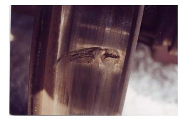
The track consists primarily of 132-pound continuous welded rail (CWR) that was manufactured and laid in 1980. There are 3200 hardwood ties per mile of track. Double-shouldered tie plates are fastened with four spikes per tie. In the derailment area, the ties were in good condition. The maximum authorized weight of the cars is 286 000 pounds. The accumulated tonnage on the track since it was laid is 450 million tons.
