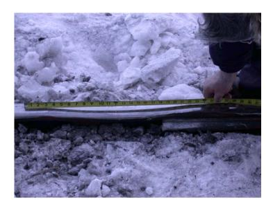
The crushed rail head was not noted in the bi-weekly inspection records. The TSR do not define a crushed rail head as a defect. It is considered a defect in SPC 3207 when the depth reaches 10 mm, but no corrective action is required.
