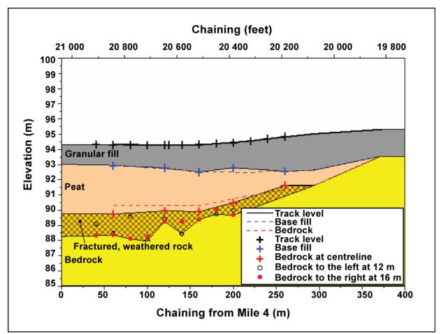
Figure 2. Longitudinal stratigraphic section
