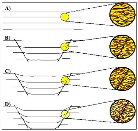
Figure 4. Evolution of settlement and distortion of peat fibres
