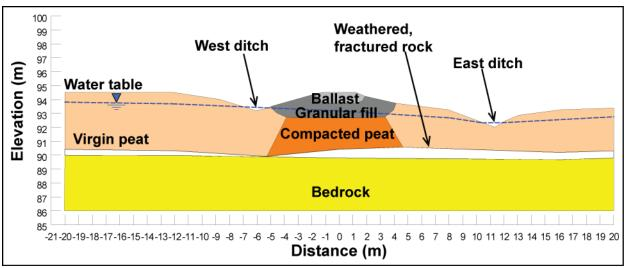
Figure 3. Cross-section at Mile 3.87
