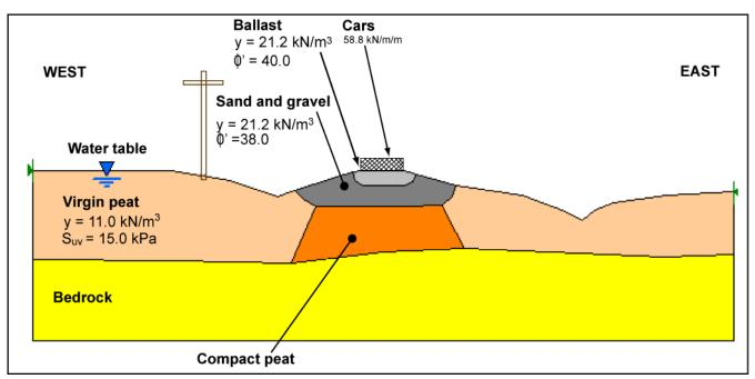
Stability of track fill slopes under the load of cars –  $s_{uv} = 10.0$  kPa for compact peat – Stable slope because the factor of safety obtained equals 1.388 ( $s_{uv}$  = shear resistance,  $\gamma$  = unit weight,  $\phi'$  = internal angle friction)
