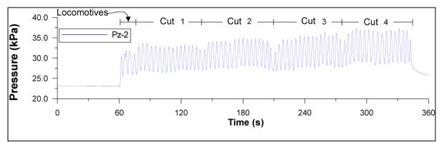
Measurement of pore pressure at the centre of the track at 3 m of depth at Mile 3.93 during the passing of a loaded train travelling at a speed of 10 mph
