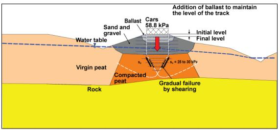
Figure 5. Shearing failure by punching at Mile 3.87
