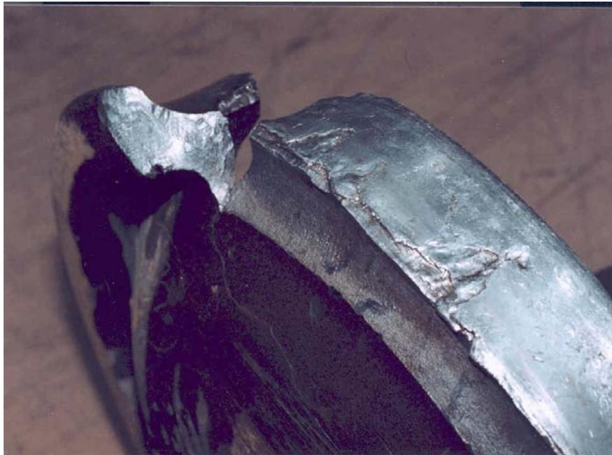
**Photo 2.** Shelling on the running surface
