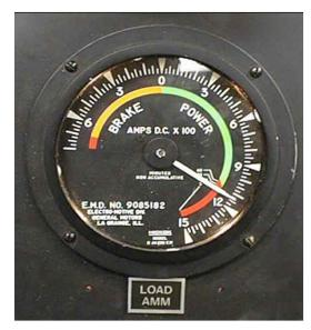
Photo 6a. Analog loadmeter display
