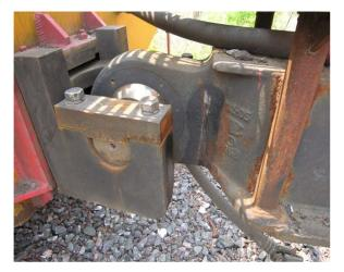
**Photo 1b.** Close-up of orbital joint showing fresh strike mark from lateral movement to limits
