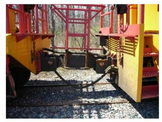
Photo 1a. Non-standard coupling system between car HZGX1750A on the left and car HZGX175 (the Herzog locomotive) on the right
