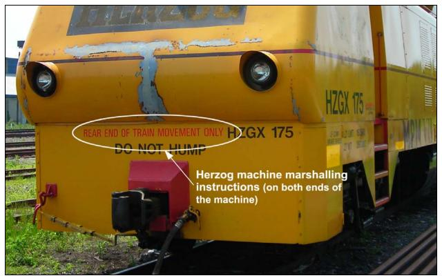
Photo 8. Herzog machine (locomotive HZGX175)
