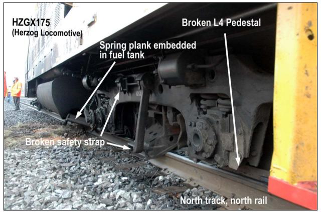
Photo 2. Damage to north side of HZGX175 (Herzog locomotive)
