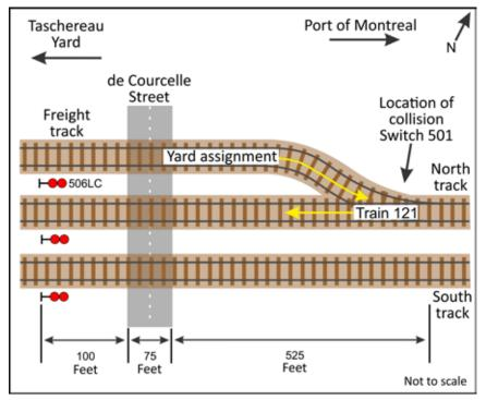
An examination of the CTC recordings revealed no operational malfunction of signals. Signal 506LC at Saint-Henri indicated a stop signal and approach signal 38E indicated "Clear to Stop."<sup>9</sup>
