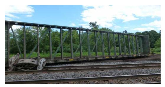
Photo 1. First derailed car, centrebeam bulkhead flat car BCOL 730558
