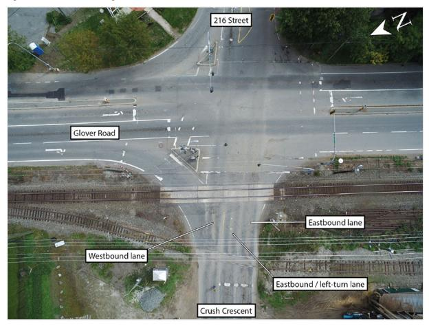
Figure 4. Faded road markings at the occurrence site (Source: RCMP, with TSB annotations)
