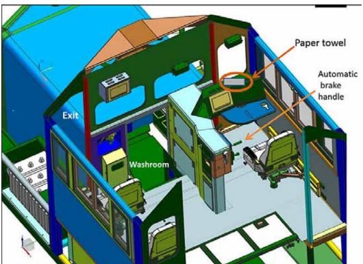
Figure 3. Locomotive cab layout
