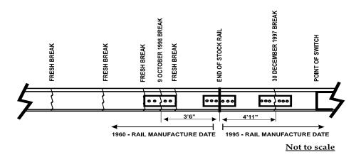
Immediately south of the crossover switch point, the rail had a previous fracture that had been observed on 09 October 1998. The adjacent rail length also had been fractured on 30 December 1997.
