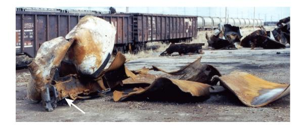
The majority of the jacket was found about 300 feet (91 m) southwest of the point of detonation. Based on the sections of trees it struck and destroyed, it was approximately 75 feet (23 m) in the air at its highest point. The jacket was hot as it flew through the air. It scorched all the wood it came into contact with as well as the ground where it landed. Some parts of the jacket showed metal thinning and stretching at failure.
